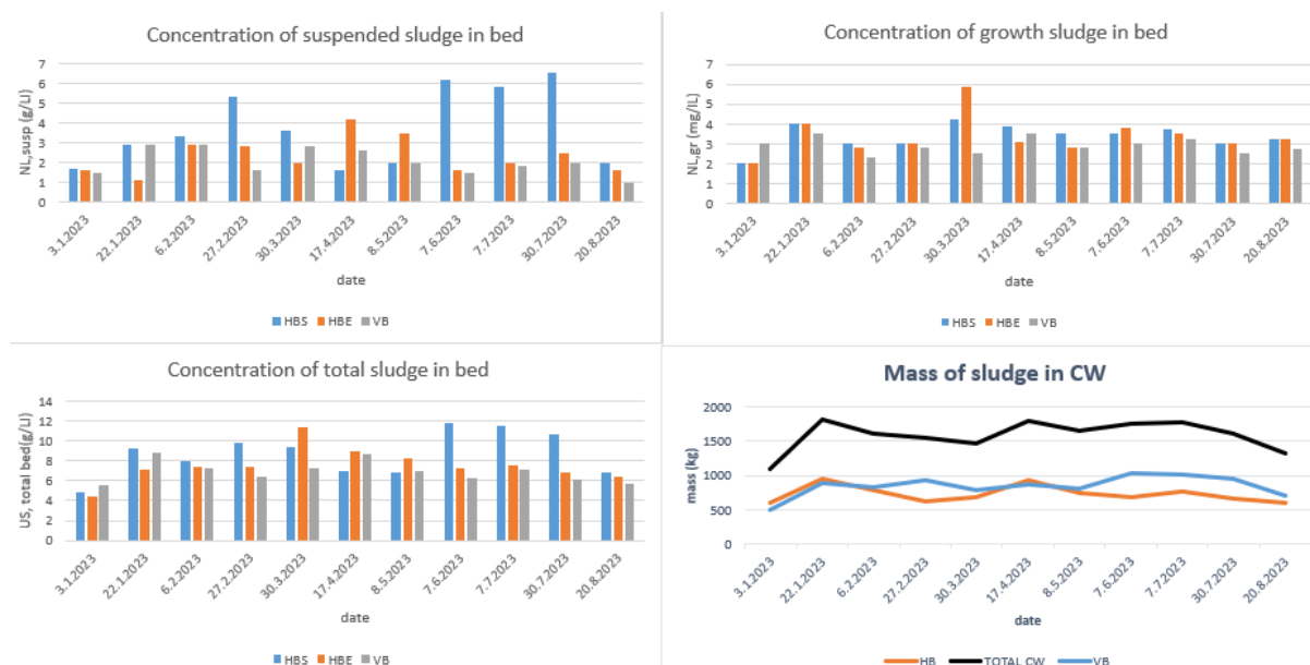
Figure 5: Concentrations and amount of sludge in CW filters
