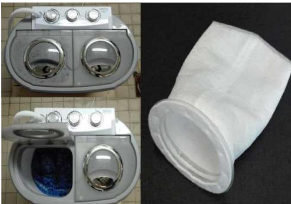
**Figure 4: The laboratory model of washing machine (Camry – CR8052) and filter (1, 25 100  $\mu\text{m}$ ) used for catching wastewater from washing machine.**
