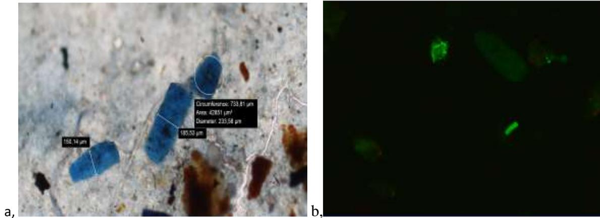
**Figure 8:** The picture of microplastics on the filters under optic (a) and fluorescence (b) microscopy after washing process (blanket 100 % PET).
