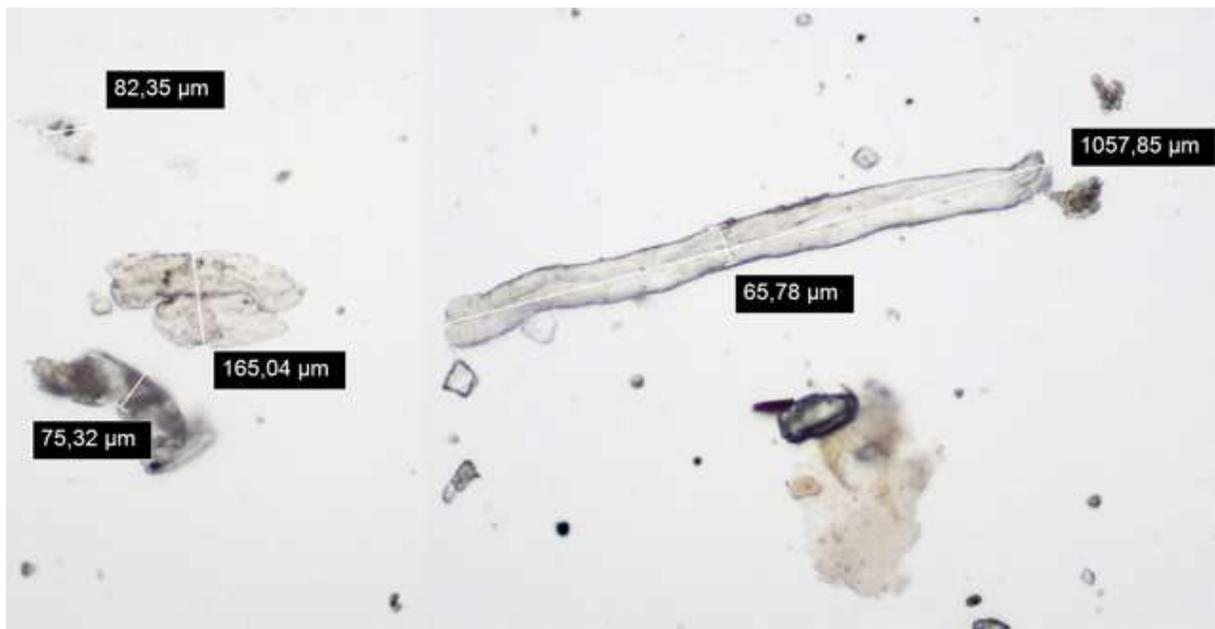
**Figure 7:** Microfibers in waste water under fluorescence microscopy from washing process (filter 100  $\mu\text{m}$ ).
