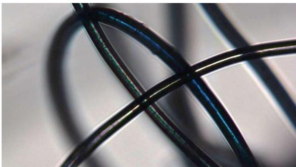
**Figure 5:** Microfiber (from blue blanket 100% PET) released during a washing process with a temperature of 40 °C and a washing time of 30 minutes.
