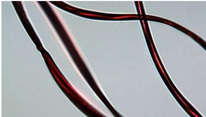
**Figure 6:** Microfiber (from red blanket 100% PET) released during a washing process with a temperature of 40 °C and a washing time of 30 minutes.
